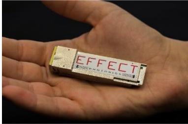
RocketChip integrated optics solutions have been developed to be compatible with physically small, and compact (small form factor) modules. The squeeze in volume and increase in speed per channel associated with small form factors bring important engineering challenges in the transceiver design. For example, more advanced assembly techniques are required and the hardware performance at higher speed needs to be guaranteed. These challenges were successfully addressed in project RocketChip.
